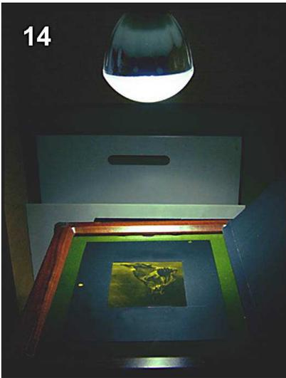
14 The paper is exposed under UV light. I use a 120 watt HPR lamp from Philips. Correct exposure has to be determined by testing; I use to expose for 4 to 6 minutes at a distance of 25cm. (pict. #14)
