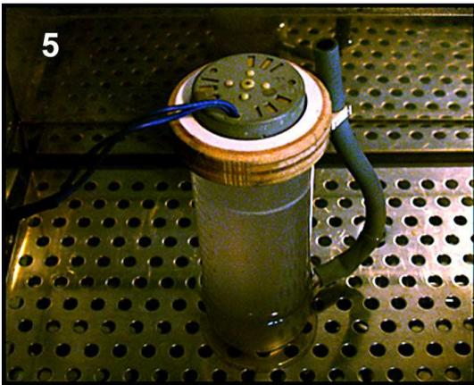
In order to avoid any air bells, I stir the solution for an hour with an automatic stirrer (pict #5).
