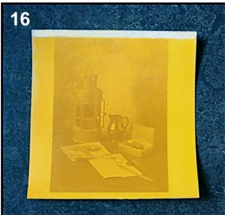
16 The UV light causes the dichromate layer to turn brown. When the highlight details in the image become just visible, the exposure is correct.
