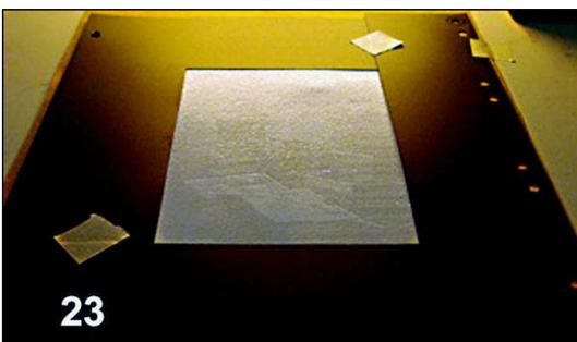
The matrix is dabbed with a sponge to eliminate the slightest trace of water on its surface.
