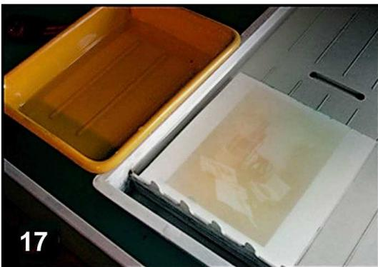
17 After exposure, the paper is washed in cold running water to remove most of the dichromate yellow stain. Any residual stain will be removed afterwards in a special bath.
