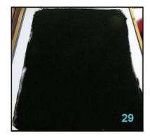
The gelatin-pigment mixture is then poured on the paper and evenly spread out with a few movements of an aluminum rod.
