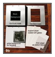
The second, somewhat simpler frame basically is a board on which four registering pins were glued. The surface was painted black. For focusing, I use a white sheet of pvc that fits on the registering pins.
