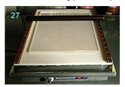
In order to make the coating easier, an accessory was built. It is composed by a plate in plexiglass on both sides of which were fixed aluminum profiles which will determine the thickness of the coat. In the middle of this is sitting a removable plexi plate on which the paper is to be laid (see picture #27).
