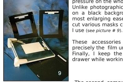
These accessories make it a snap to position precisely the film under the enlarger.
