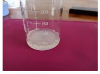
> Put the beaker in a water bath at 42°C and leave it there for at least 30 minutes. The gelatine will liquify. Some impurities may be visible in the beaker. The settling time is intended to reduce the presence of microbubbles in the mixture.
