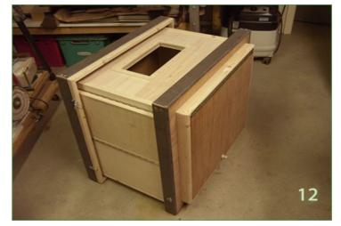
The front and rear panels are maintained against the body of the box by tension cords; foam sealing strips allow for light-tightness. *See picture 21*.
